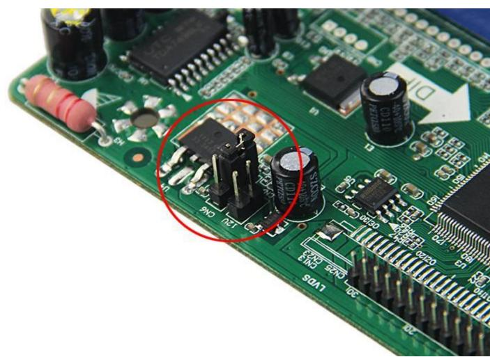
\* link the key button board, (starts from left side, and leave some pins on the right blank), and connect inverter with controller
