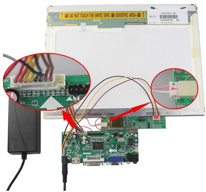
\*According the above operated way , then unplug the power supply, Connect LV DS with the LCD connector and control board
