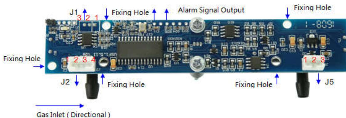
**Drawing1 Gasboard-7500E Pin Definition**
