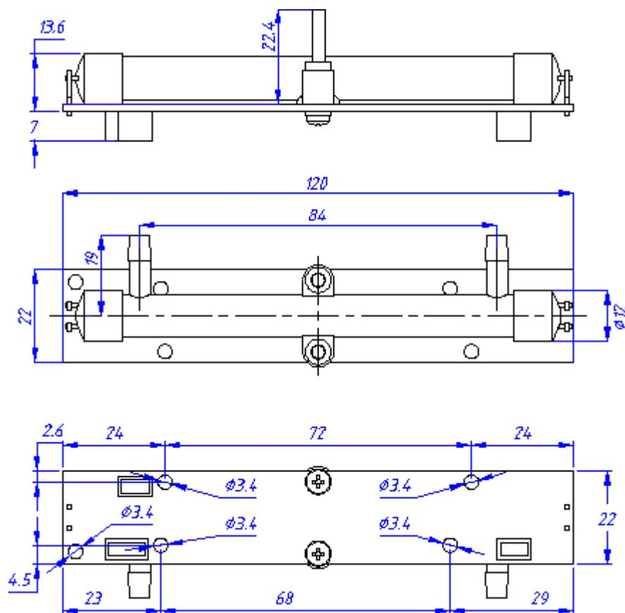
**Drawing 3** (Unit:mm, Tolerance: $\pm 0.2$ mm)
