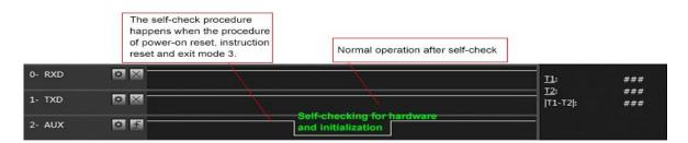
Timing Sequence Diagram of AUX when self-check
